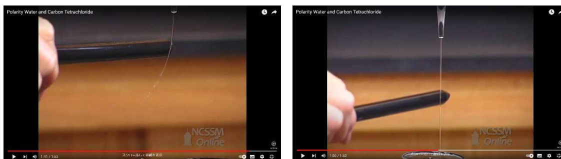
Figure 3. Flow of water (left) and carbon tetrachloride (right) near a charged rod Copyright North Carolina School of Science and Mathematics, licensed under Creative Commons CC
