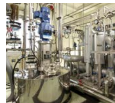
Ultra Low Temperature Reactors (-80 °C, 200 L)
